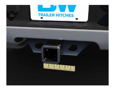
Remove any reducer sleeves (smaller tubes) from the receiver tube and measure the opening as shown. Using reducer sleeves can decrease the tow rating of your hitch and create additional noise while towing.
